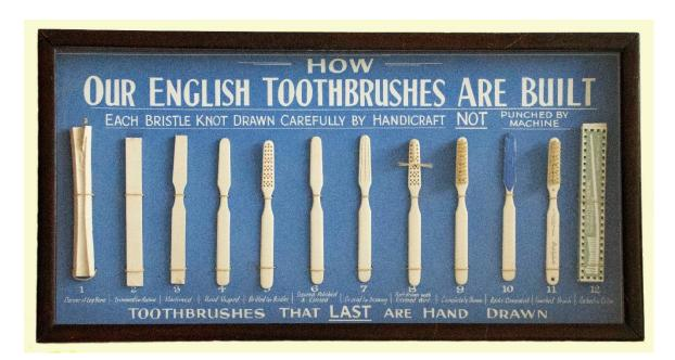
The case shows 12 stages of development from raw bone, through trimming and machining to shape, followed by polishing and drilling, then pulling the bristles through and cementing the back to hold the bristles in place. Finally, we have the finished brush and an example of the packed brush in a carton.
